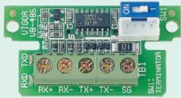
RS-422/RS-485 Communication Expansion Card VB-485
